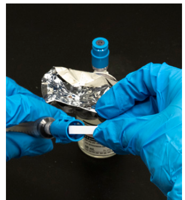
Testing ChemoLock injector with wet litmus paper
