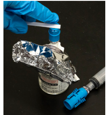
Testing ChemoLock port with wet litmus paper
