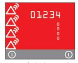
System fault alarm (red). The numbers relate to the error that caused the system fault.
