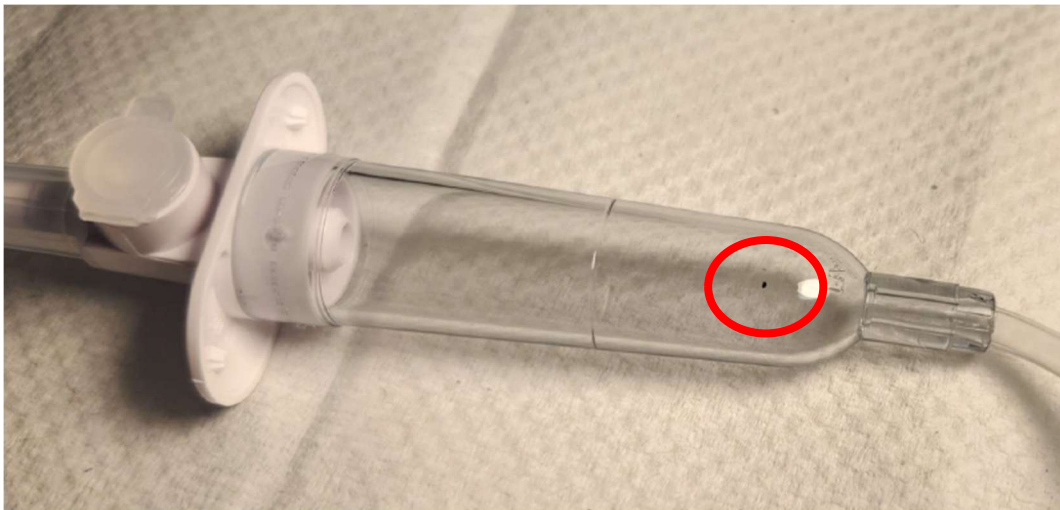
Figure 1: Embedded black speck in the wall of the drip chamber from healthcare provider
