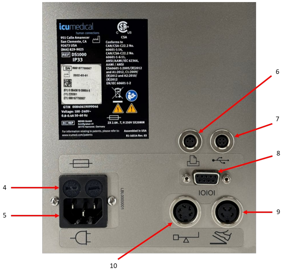
Figure 4. Back of the Pump Unit
