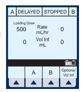
After the programmed delay period has expired, the Plum A+ starts "Pumping". This is indicated where "Delayed" previously was displayed.
