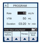
shown in this example, the delivery shows 3 hours and 20 minutes (not 3 minutes and 20 seconds).
