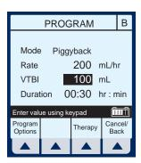
At end of Piggyback delivery, with Callback enabled for the line, Callback alarm is issued.
