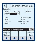
**NOTE:** The Concentration elements and weight value must be entered before the [SELECT] keys allow access to remaining fields.
