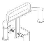
Always mount the tandem carrier (List# 12270-01) to the pole before attaching the infuser(s) to the tandem carrier.
