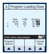
11) After the values for loading dose (Step 1) are entered, use ▼ to highlight the maintenance dose, (Step 2).
