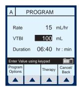
**NOTE:** When the VTBI is changed, the Duration is recomputed with respect to the current Rate. To understand the Automatic Calculation feature, *see "Examples of Automatic Calculation" on page 6-14.*
