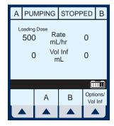
After the Step 1 (loading dose) has completed, the Main Delivery screen changes to the second step (maintenance dose).
