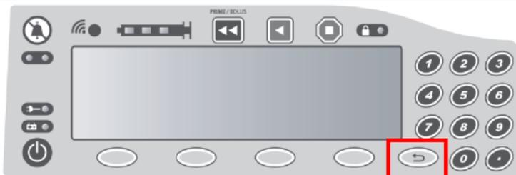
4) If you miss the size on the screen, pressing the back button on the pump will again briefly flash the size of the syringe in the upper left hand corner without stopping the infusion. The screen will then return to the normal run screen.
