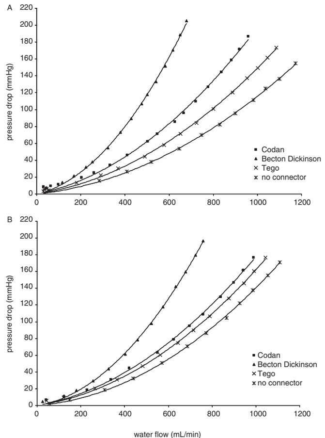
**Fig. 1.** Measurement results (symbols) of pressure and water flow in different types of connectors and without any connector for venous flow (catheter inflow) (Panel A) and arterial flow (catheter outflow) (Panel B).
