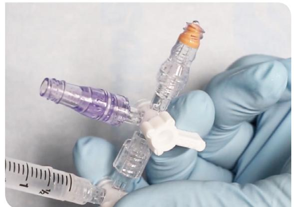
product performance is not in line with generally accepted performance guidelines in regard to back pressure.\* Pressures like these are common in clinical practice and are easily demonstrated with a simple stopcock and a standard three mL syringe (see Figure 3).
