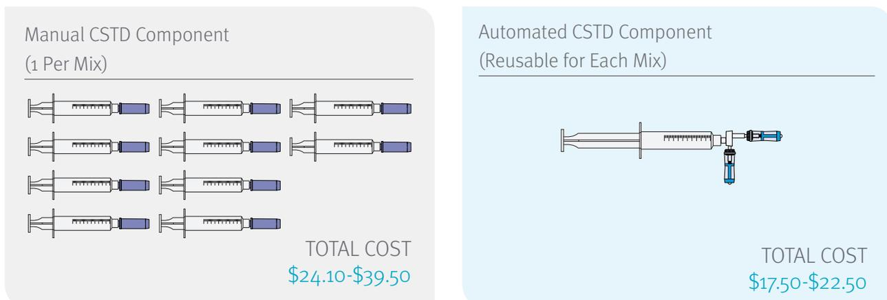
The Diana system integrates a reusable CSTD component that transfers HD from a vial into a patient IV bag or syringe. As a result, this reusable component replaces the need for single-use syringe adapters that would normally be disposed of after each use, allowing the cost per mix of CSTD disposables to decrease the more times the system is used (Figure 3).
