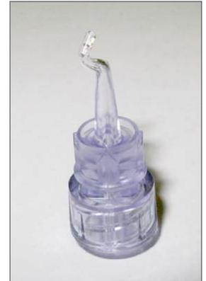
Pictured is a MicroClave spike that has been damaged by the Texium closed male luer. The spike should be straight and this damage could lead to possible leaks.
