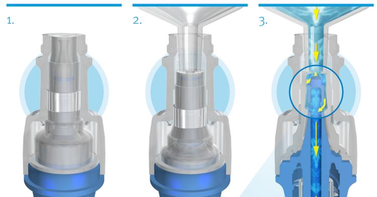
The male luer depresses the silicone, forcing it against a rigid internal column which spreads the pre-split septum. The rigid column incorporates four channels to allow fluid flow around the spike, into the silicone, then into the windows of the spike.
