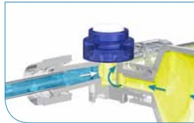
By simply pushing the button of the 1o2, it converts to a two-way valve that permits aspiration. When the button is released, the 1o2 valve automatically returns to the closed one-way position. The sideport aspiration feature is useful to prime the 1o2, dilute a drug, draw a flush syringe, or conduct a blood draw.
