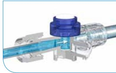
The valve sideport port allows for intermittent drug delivery with the security of a one-way check valve. This pressure activated one-way valve protects the system from accidental infusion, or the mixing of incompatible drugs and fluids on a manifold. Propofol, Lipids and Blood products can safely be administered through the 1o2 valve.
