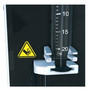
3.6.1.4. To Connect Drug Vial (Input Container) to Syringe Cassette: Invert vial containing the Chemolock vial access device to the vertical Chemolock connector on the Syringe Cassette.
